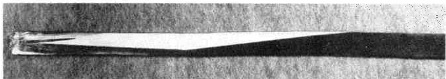
Figure 7a. The growth competition of crystals in a Sn plate.
