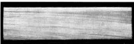
Figure 6a. Striations in a Sn plate; 60 mm/min.
