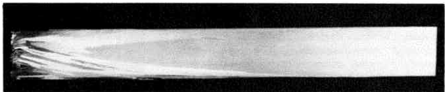
Figure 7b. The growth competition of crystals in an Al plate.
